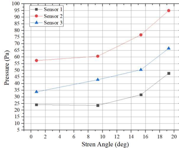
**Figure 12.** The value average of the pressure in each variation of the stern angle.
