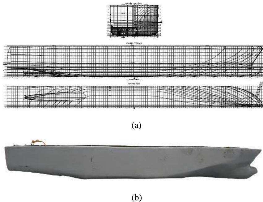
**Figure 4.** (a) Lines plan Ship Ferry ro-ro and (b) Model Ship Steel
