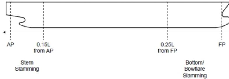
**Figure 2.** The extent of hull structure for slamming
