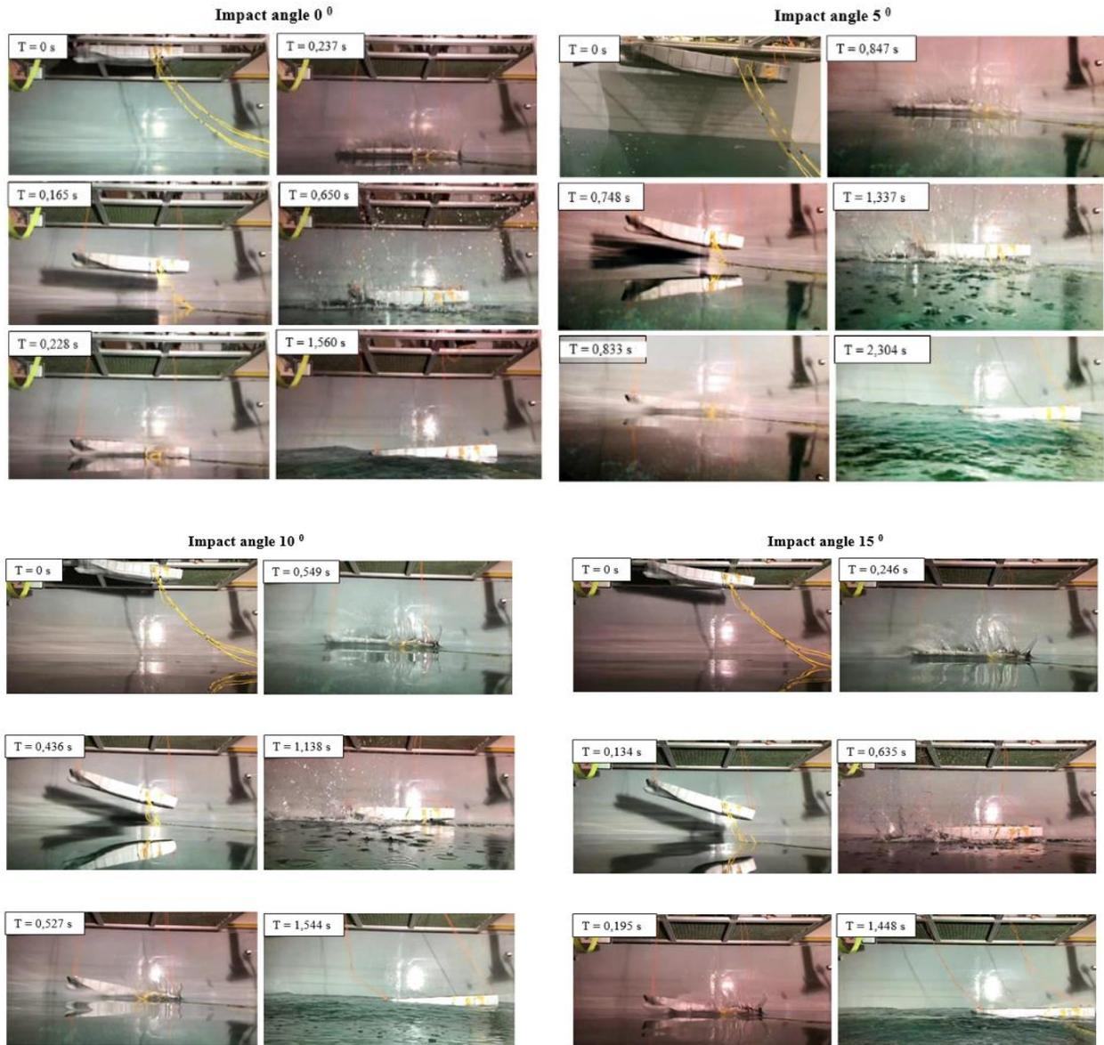
**Figure 10.** Snapshots of the ship model during the dropping test.
