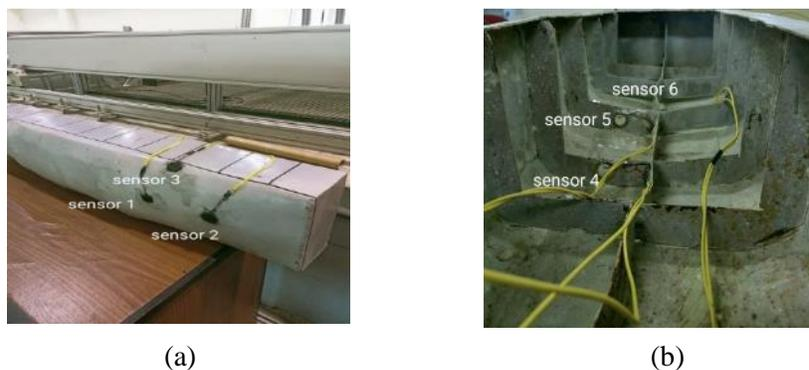
**Figure 9.** (a) Sensors on the bottom stern (b) sensors on the frame on the construction.
