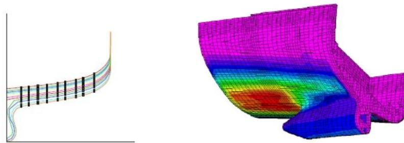
**Figure 3.** Typical frame section location for stern slamming
