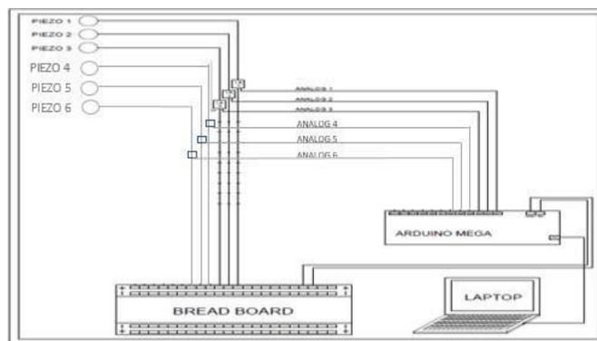
**Figure 7.** Block diagram of piezoelectric device circuit.
