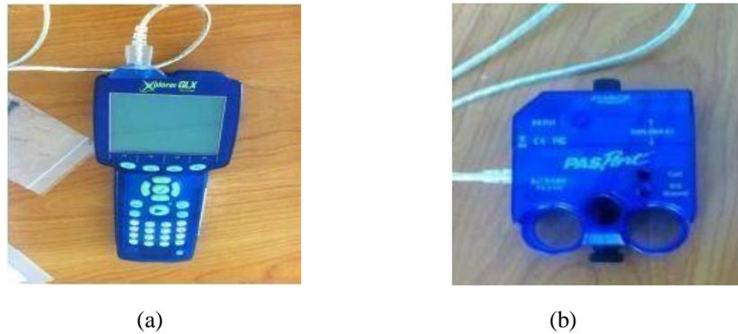
**Figure 8.** (a) Xplorer GLX and (b) Force sensor
