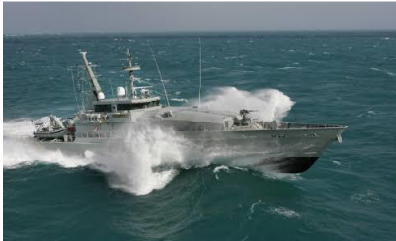
Figure 1. Slamming Phenomena (Veen, 2010 [2])
