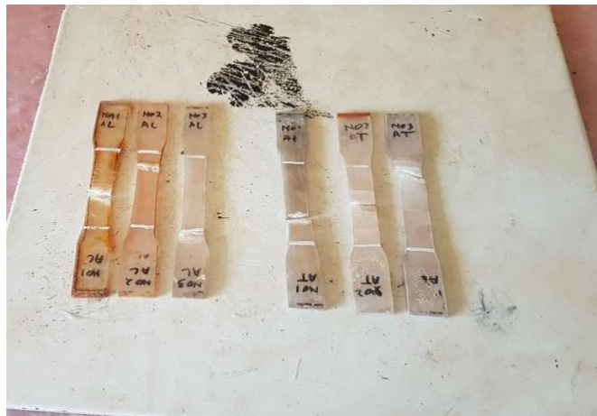
Figure 11. Fracture of composite tensile test specimen.
